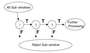
Figure 2. Schematic of cascade classifier [14].
