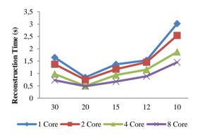
Figure. 13. A graph showing the Time Complexity of reconstructing Phantom image of size 64x 64 sequentially, parallel in 2, 4 and 8 core with respect to projections.
