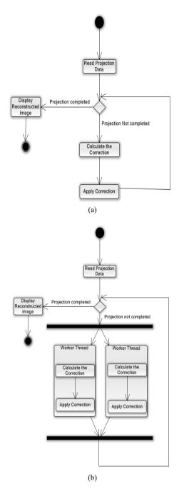
Figure. 8. UML Activity for reconstructing an image using ART. (a) Sequentially (b) Parallel
