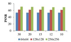
Figure. 11. Plotted the PSNR value obtained while reconstructing Shepp Logan Phantom Images on 64x64, 128x128 and 256x256 sizes using 30, 20, 15, 12 and 10 number of projections.
