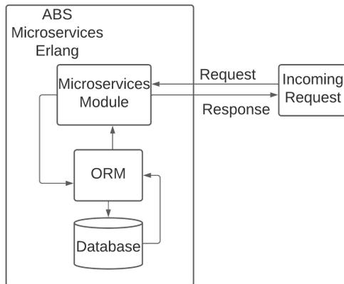
**Figure 2.** ABS Microservices Erlang Design
