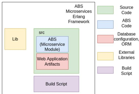
**Figure 5.** ABS Microservices Erlang Directory Structure
