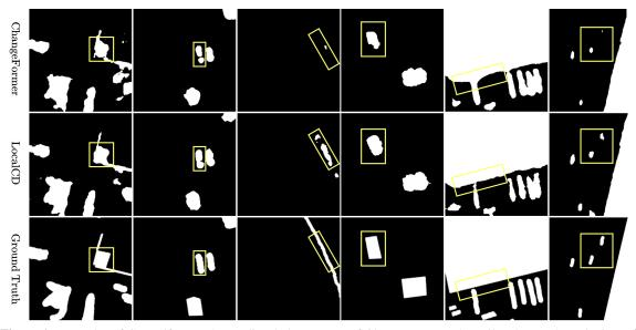
Figure 1. Examples of CD artifact on the predicted change map of ChangeFormer. The yellow boxes show the imperfect changed region boundaries.
