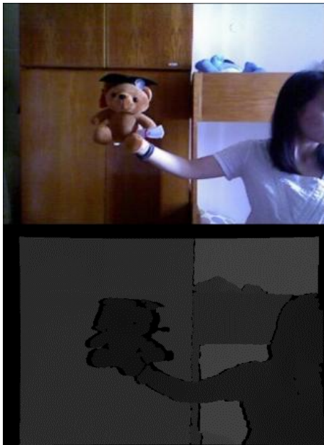
Fig. 4. Paired RGBD image: RGB(Above) and depth (Below)
