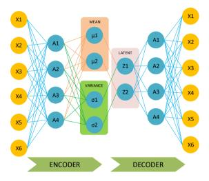
Figure 2. Basic structure of Variational Autoencoder (VAE)
