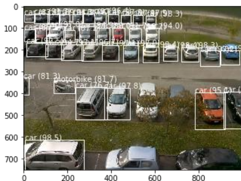
Figure 5. Result of the marking stage using YOLO V3 and create a bounding box on each car.
