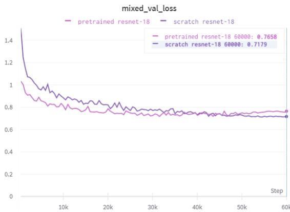
Fig. 7. Comparison of scratch ResNet-18 with pre-trained ResNet-18 validation loss graph
